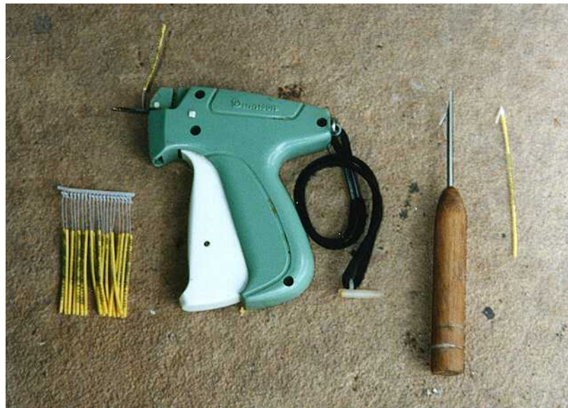
Figure 1: Left to right – clip of anchor tags – tag gun – dart tag applicator – dart tag
