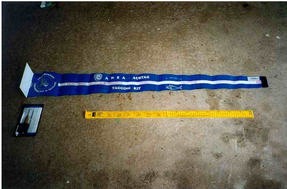
Figure 2: top – roll up fish measure – lower left – dart tag tagging kit – lower right – fold up tag ruler
